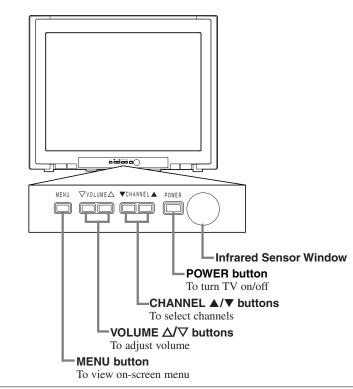
• If some digits appear in the corner of the screen when the unit is turned on for the first time, press **[POWER]** without unplugging the power cord.
